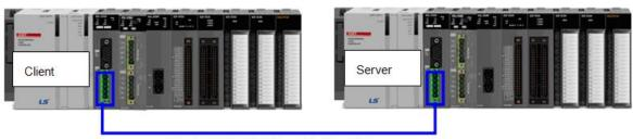
\* RS-422 38400/8/1/None/Modbus RTU
