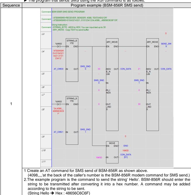
3.30 data of SMS\_SND0 and 21 data of SND1 are saved to variable CON\_DATA[51] in bytes.
