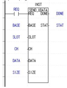
Command that transmits up to 1024 bytes using the Cnet I/F module installed on BASE and SLOT
