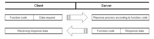
If the Modbus communication is abnormal, the server transmits the response, including the error code, to the client, as shown in the figure below.
