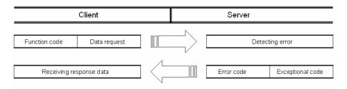
When an abnormal frame is received, the server transmits the error code and the exception code to the client. The error code is the value of the function code plus 80(Hex) value, and the exception code indicates the error details. The contents of each code are as follows.
